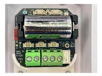
Connector: **LED** 3 separate LEDs or RGB LED
